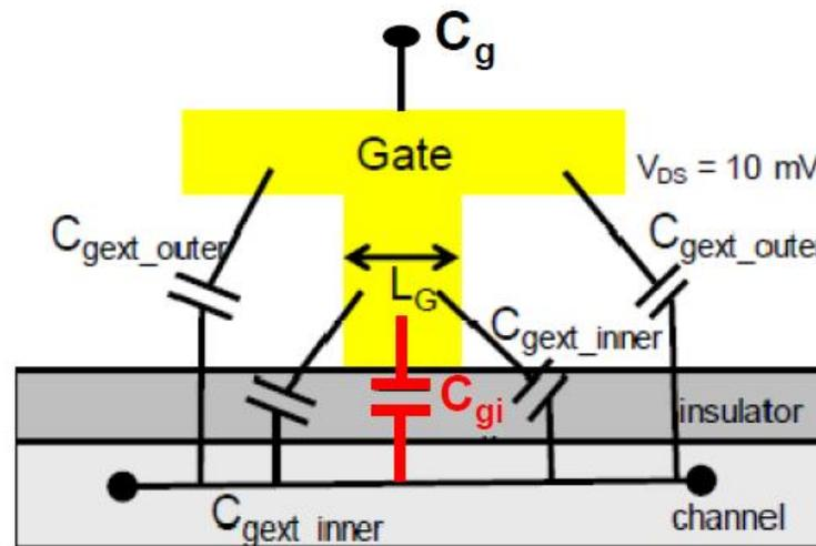
$$C_g = \underbrace{C_{gi} \times L_g + 2C_{gext\_inner}}_{\propto f(V_{GSI} - V_T)} + \underbrace{2C_{gext\_outer}}_{\approx C_g @ \text{OFF}}$$
