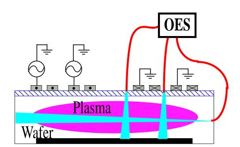
Figure 5-1: Optical emission spectroscopy experiment setup
